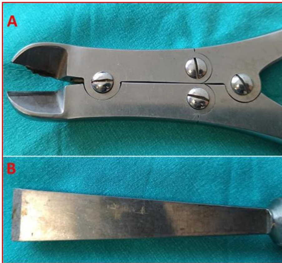
Figure 1. (A) A bone/nail cutter with a broken mouth and (B) a fractured and corroded osteotome
